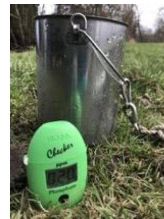
Figure 21: P results from sites sampled using the Hanna HI-713 digital photometer checker (Wensum P target = 0.05 mg/l)
