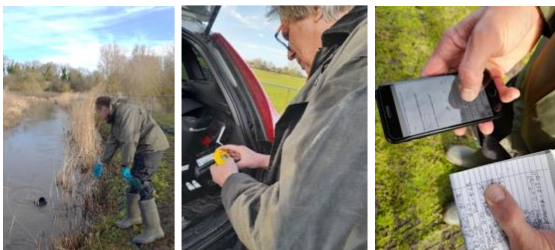
Figure 20: (L-R) – Taking a water sample from the Wendling Beck at Worthing Fishery; Colin Howlett undertaking ammonia testing using the Hanna HI-715; uploading site data onto the mWater app
