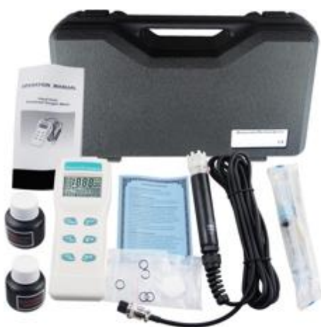
Figure 13: AZ instruments 8403 digital dissolved oxygen meter
