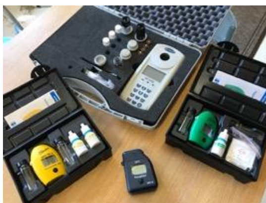
Figure 18: Comparing low-cost digital photometers against the Lovibond MD610
