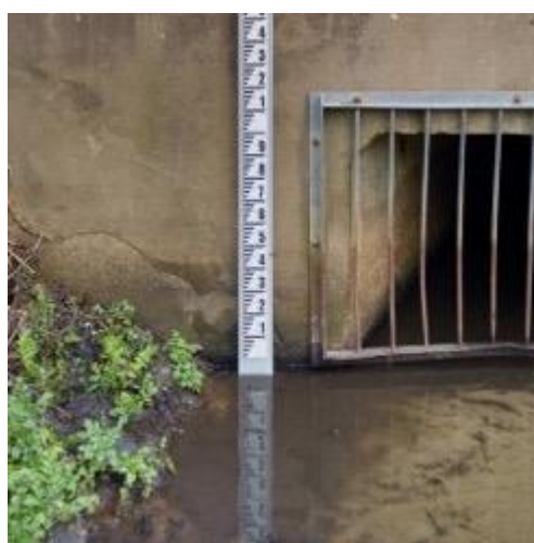
Figure E4: Fixed point photographs can capture river levels and also evidence other impacts such as sediment-rich run off smothering river beds after intense rainfall events (bottom right of picture)
