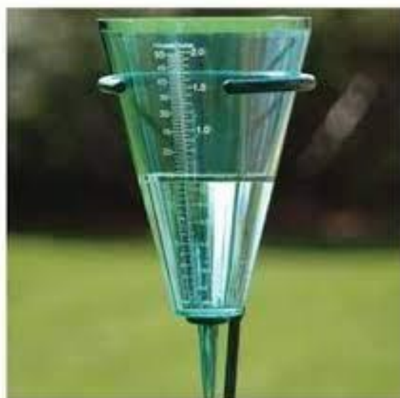
Figure E1: Example of a simple rainfall gauge for monitoring precipitation
