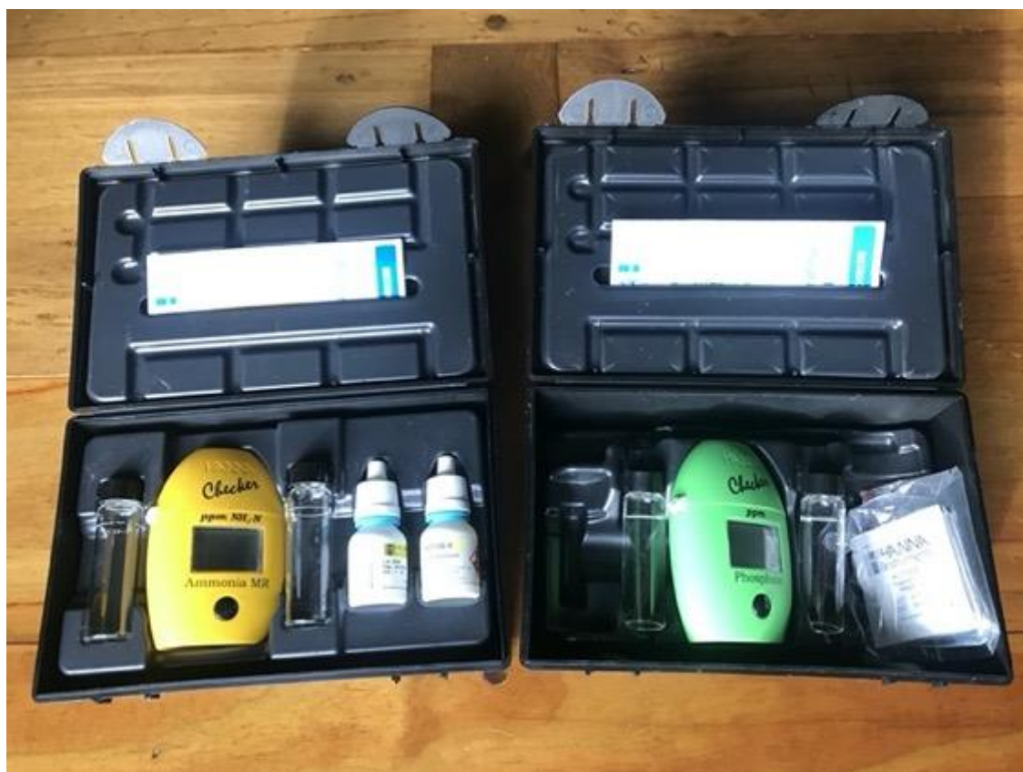
Figure D1: Hanna HI-715 Medium Range Ammonia and HI-713 Low Range Phosphate Checkers
