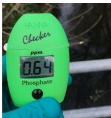
Figure 12: Low-cost digital photometers such as the Hanna Phosphate checker HI-713 and the Milwaukee MW12 can give a digital readout of sample test results to \pm 0.01 mg/l resolution
