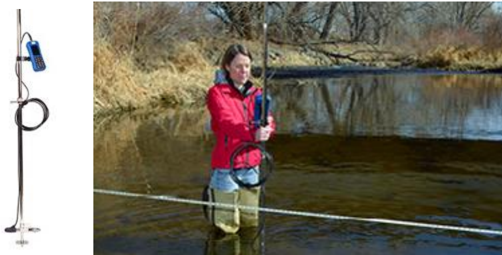
Figure E13: Measuring stream flow with the OTT MF Pro flow meter (Source: OTT)
