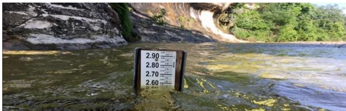
Figure E3: Example of a fixed stream gauge to record river levels (Credit: USGS)
