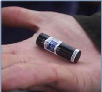
250 Internal acoustic transmitters emit coded 'ping'
